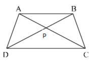
In ΔAPB and ΔCPD, ∠APB = ∠CPD .....(vertically opposite angles) ∠ABP = ∠CDP .....(alternate angles since AB||DC) ∴ ΔAPB ~ ΔCPD ....(AA criterion for similarity)
