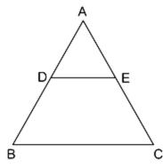
Since DE || BC,  $\triangle ADE \sim \triangle ABC$  $\Rightarrow \frac{AD}{BD} = \frac{AE}{EC}$   $\Rightarrow \frac{AB - BD}{BD} = \frac{AE}{EC}$   $\Rightarrow \frac{5BD - BD}{BD} = \frac{AE}{EC}$   $\Rightarrow \frac{4BD}{BD} = \frac{AE}{3.2}$   $\Rightarrow AE = 4 \times 3.2 = 12.8 \text{ cm}$
